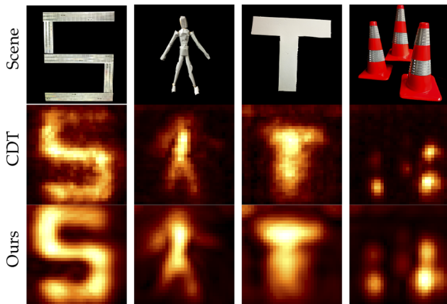
Fig. 6. Reconstructions of experimental data. Each column is a different scene. Top: images of the scenes behind the diffuser. Middle: Lindell and Wetzstein reconstructions [21] (CDT). Bottom: our reconstructions using phasor fields . The higher frequency of CDT is related to the deconvolution to compensate scattering at the diffuser.
